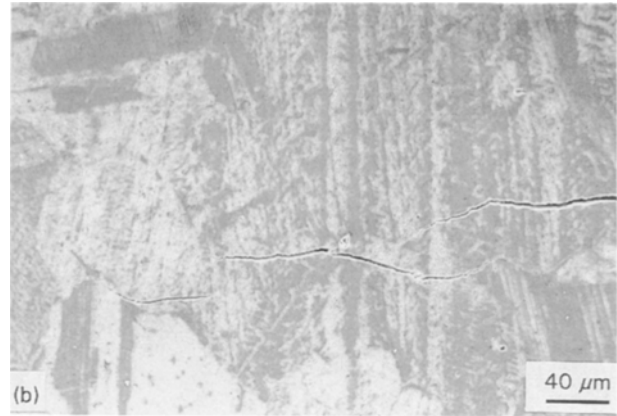
Figure 8 Fracture crack path morphology of test materials. (a) Microcracking and bridging in HT-TiAlCr; (b) uncracked ligaments in HT-TiAlCr; (c) crack branching in ITF-TiAlCr.
